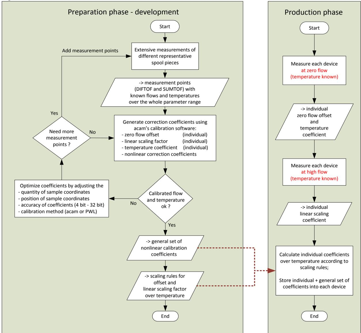
Within this document, we assume that the characterization of the spool piece design in development was done, and a general set of calibration coefficients is available as firmware data file (reference calibration). Note that of course characterization in development and later measurements of production devices have to be done with identical configuration settings to avoid
