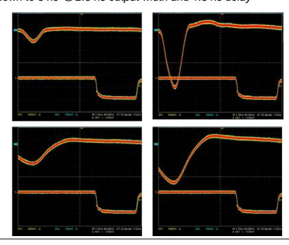
Fig. 1: CFD operation for various pulse amplitudes and shapes
